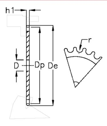
C = 1 D = 16 De = 110 Dp = 105.36 For chain size = 1/2 x 5/16 For chain type = 08 B-1 h1 = 7.2 Solution Number of teeth = 26
